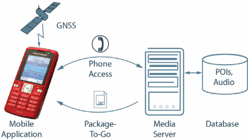
Figure 3. Architecture and concept of the MontaPhone communication
