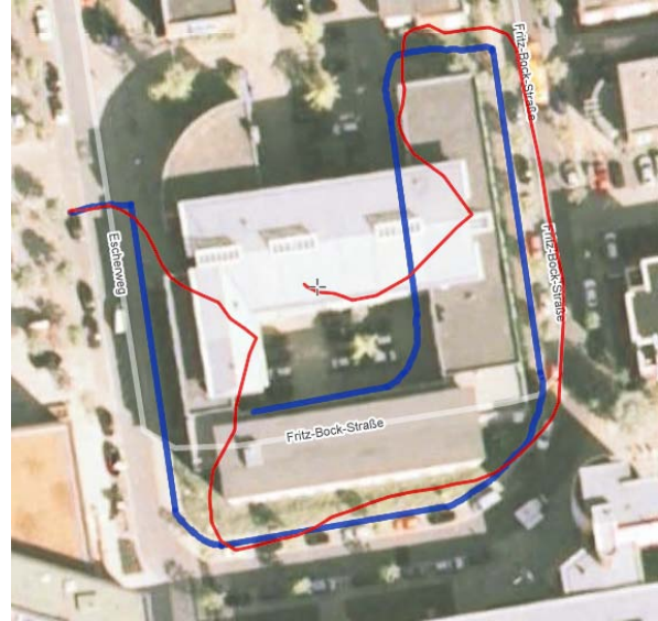
Fig. 2. Dislocation near buildings and walls
